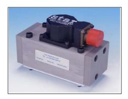
2-stage mechanical feedback Low mass, high band-width torque motor High spool drive forces Long life "Sapphire Technology" design High resolution, low hysteresis Rated flows 95 to 125 l/min at 70 bar Internal pilot supply (4 port) ISO 10372 size 4
