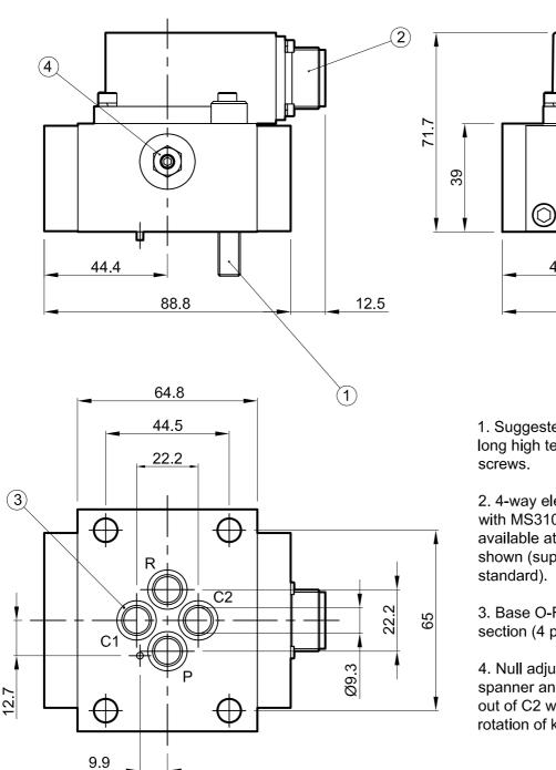
1. Suggested mounting bolts M8 x 60 long high tensile steel socket head cap
