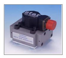
2-stage mechanical feedback Low mass, high band-width torque motor High spool drive forces Long life "Sapphire Technology" design High resolution, low hysteresis Rated flows 4 to 20 l/min at 70 bar Very-High Response Internal pilot supply (4 port) ISO 10372 size 4
