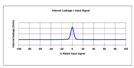
This comprises of both 1st stage flow (tare leakge) and the second stage null leakage.
